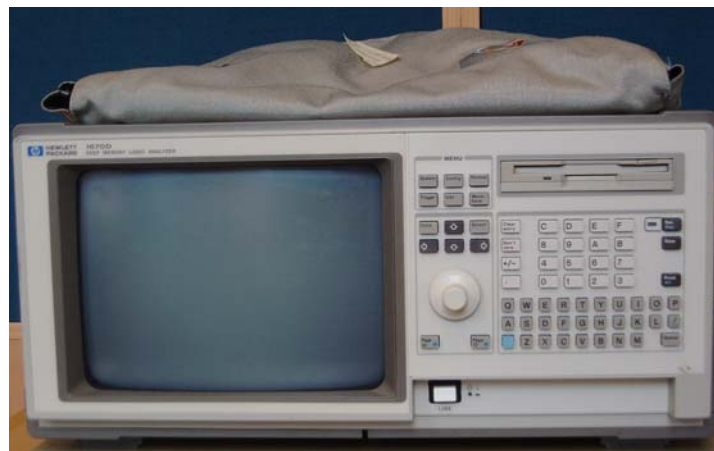
Figure 3.1.2: a typical logic analyzer made by Hewlett-Packard
