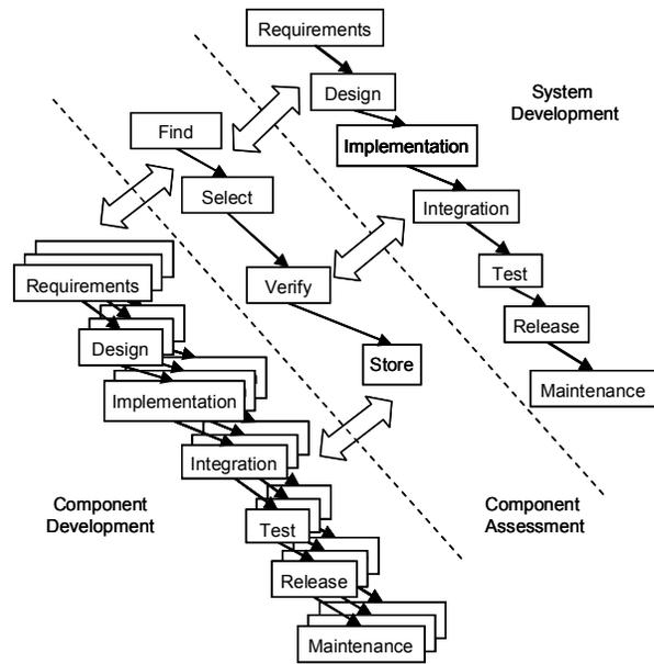
Figure 3: Parallel processes of component-based development
