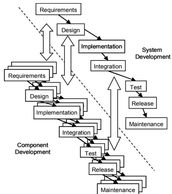
Figure 5. Architecture-driven component development process
