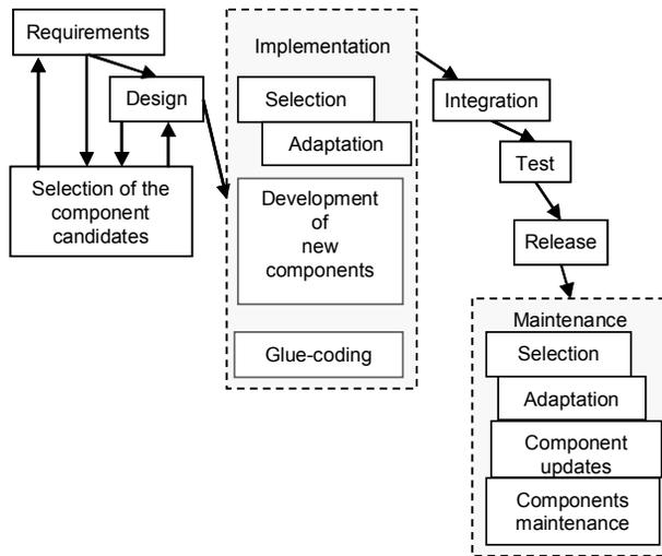
Figure 2: Component-based Waterfall Software product lifecycle
