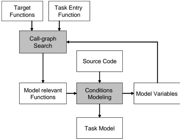
**Figure 1. The source code modeling process**
