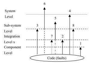
Figure 2. Fault propagation to failures, can be captured at different levels
