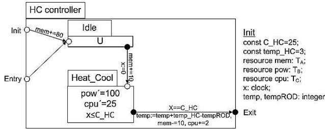
**Figure 6. The HC Controller modeled in REMES.**
