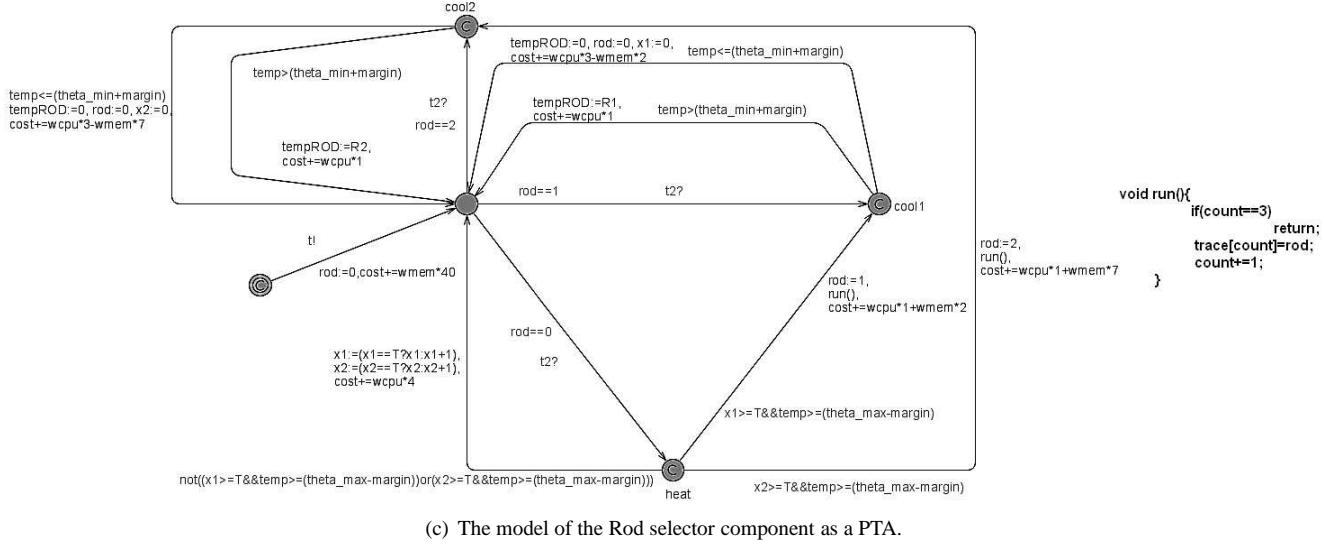
(c) The model of the Rod selector component as a PTA.
