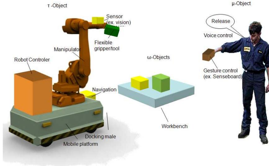
**Figure 2.** Sample cell environment demonstrating the  $\mu$ -Object as the user giving commands to the  $\tau$ -Object, in this case the robot. And a set of  $\omega$ -Objects on the workbench.
