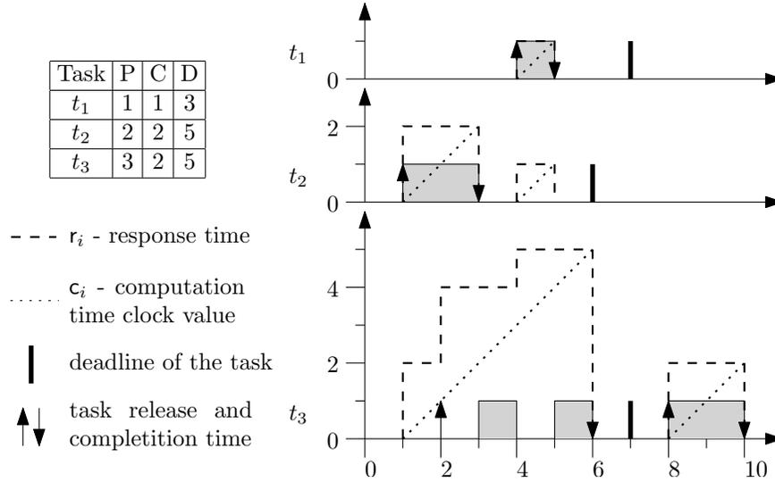
**Fig. 3.** Tracking of essential variables for each task.
