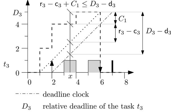
Fig. 4. Visual explanation of the schedulability predicate encoding.
