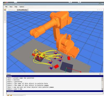
Fig. 2. Screenshot of the simulator where the robot is asked to pick and place all the blue objects into palette gamma
