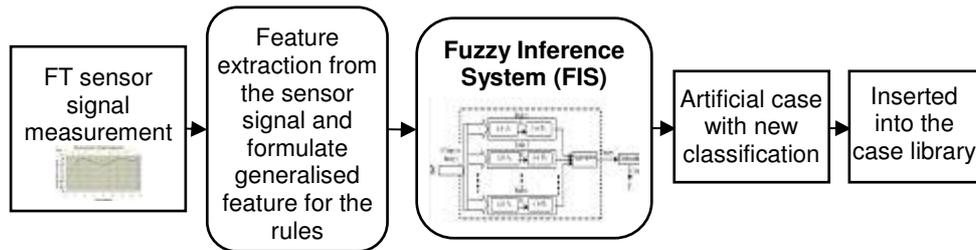
**Figure 16.** Steps to create artificial cases in a stress diagnosis system.
