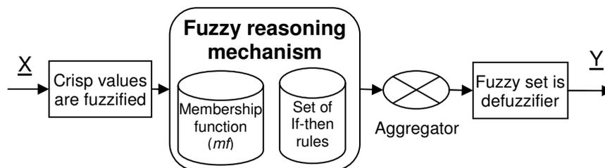
**Figure 17.** A block diagram of a fuzzy inference system [30].
