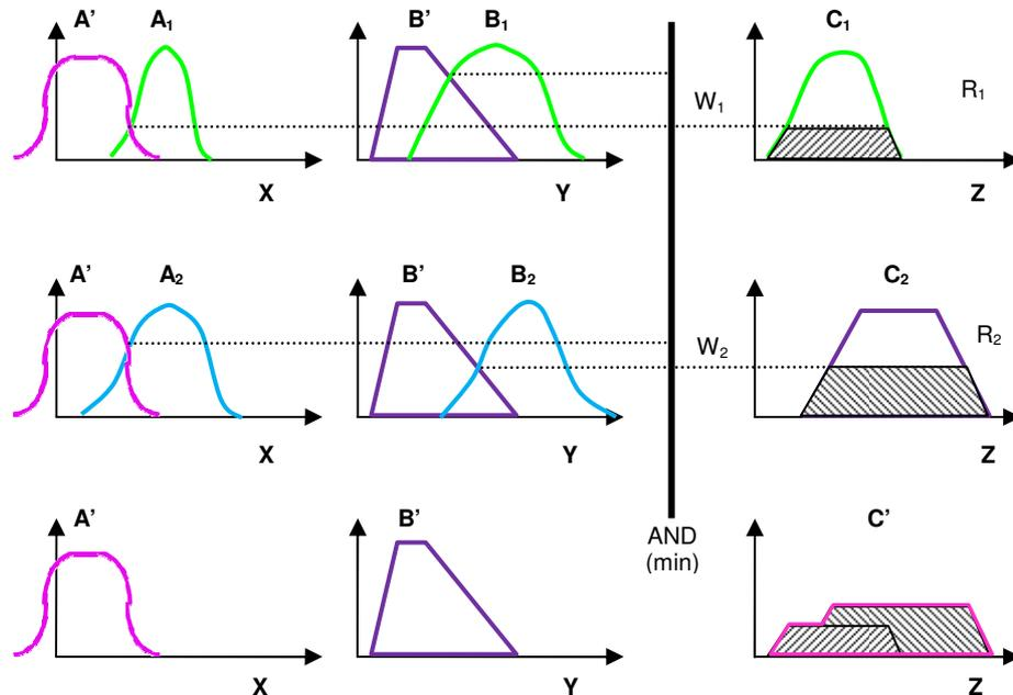
**Figure 6.** Graphical representation of an example of fuzzy inference.
