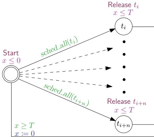
Fig. 6. A universal automaton for scheduling a task with  $n$  fallback tasks.
