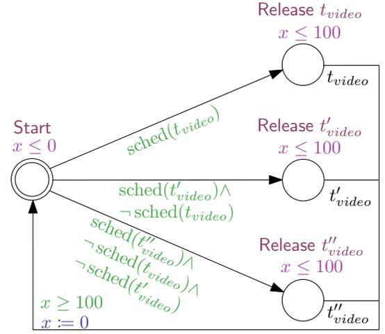
Fig. 5. Adaptive task automaton model for the user console.
