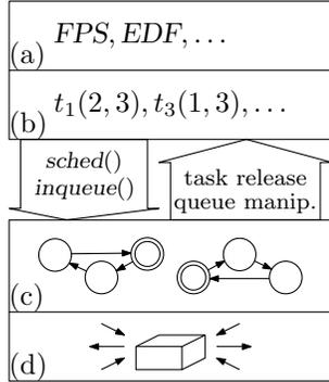
Fig. 2. Essential components of the ATA model: (a) the task scheduling policy, (b) the task queue, (c) task automata network modeling task release patterns, and (d) model of the environment.
