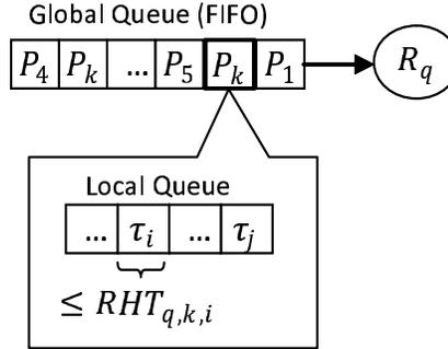
Figure 8.1: An overview of MSOS. The processor at the head of a global queue receives the corresponding global resource and within the processor the eligible task in the local queue is granted to access the resource.
