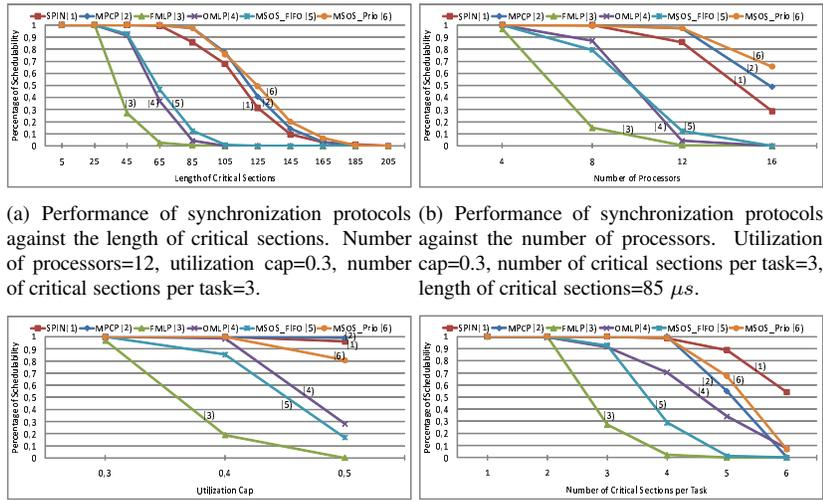
(a) Performance of synchronization protocols against the length of critical sections. Number of processors=12, utilization cap=0.3, number of critical sections per task=3. (b) Performance of synchronization protocols against the number of processors. Utilization cap=0.3, number of critical sections per task=3, length of critical sections=85  $\mu s$ .
