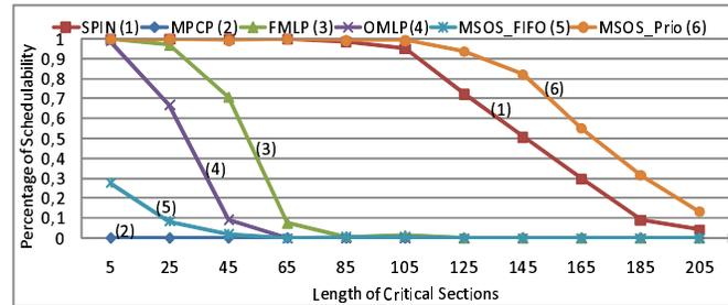
Figure 9.5: MSOS-Priority outperforms spin-based protocols in many cases for lower per-preemption overhead, e.g., as the length of critical sections is increased. Number of processors=16, utilization cap=0.3, number of critical sections per task=2, per-preemption overhead=140 $\mu$ s.
