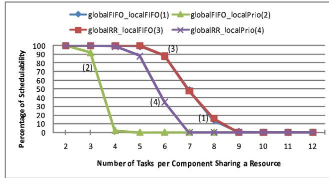
Figure 10.5: Schedulability of C-MSOS by increasing the number of tasks per component per resource. 12 component, 3 processor per component, 8 global resources each shared by 4 components, up to 4 critical sections per task each with length of 40  $\mu s$ .
