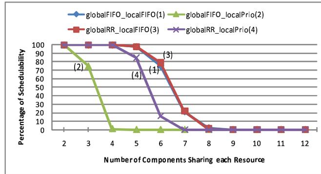
Figure 10.4: Schedulability of C-MSOS by increasing the number of components sharing each resource. 12 component, 3 processor per component, 3 global resources each shared, 4 tasks per component sharing a global resource, up to 4 critical sections per task each with length of 40  $\mu s$ .
