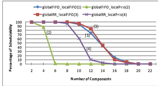
Figure 10.3: Schedulability of C-MSOS by increasing the number of components on the platform. 3 processor per component, 8 global resources each shared by half of the components from which 4 tasks share the resource, up to 4 critical sections per task each with length of 40  $\mu s$ .
