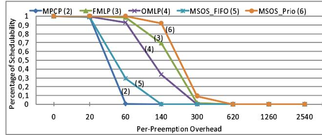
Figure 9.4: Performance of synchronization protocols as the preemption overhead increases. Number of processors=12, utilization cap=0.3, number of critical sections per task=3, length of critical sections= $25 \mu s$ .
