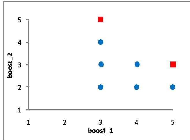
Figure 11.3: The possible allocations of boosting levels for resources. The allocations shown in squares are Pareto-optimal allocations.
