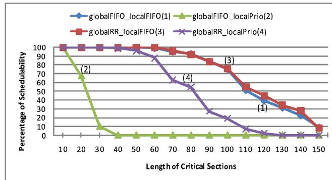
Figure 10.6: Schedulability of C-MSOS by increasing the length of critical sections (in  $\mu s$ ). 12 component, 3 processor per component, 8 global resources each shared by 4 components from which 4 tasks share the resource, up to 4 critical sections per task.
