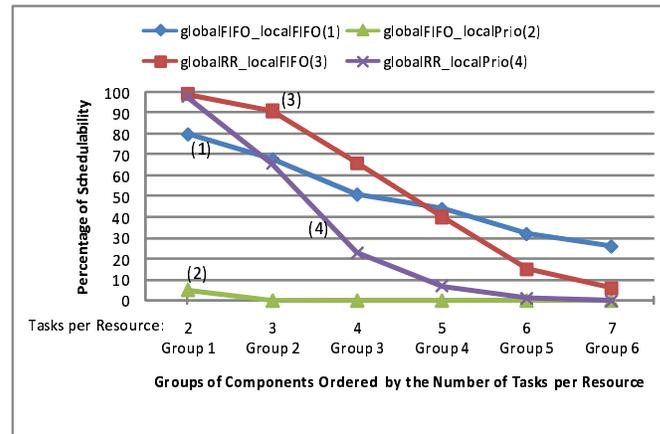
Figure 10.7: Schedulability under C-MSOS for components with different number of tasks per resource. 12 component, 3 processor per component, 8 global resources each shared by 6 components, up to 4 critical sections per task each with length of  $80 \mu s$ .
