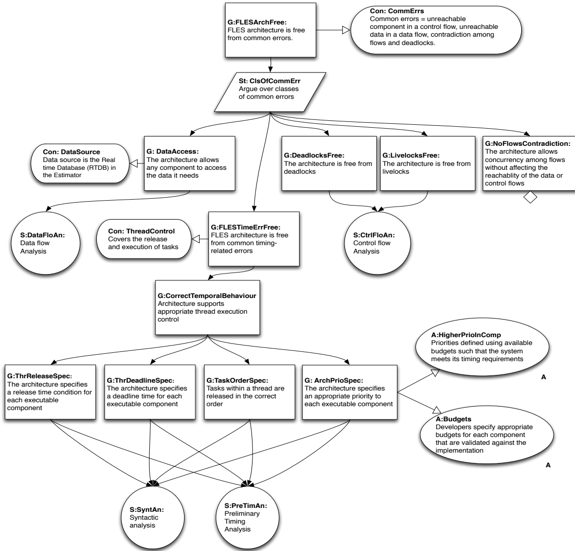
Figure 4 — Conformance Argument (Arch. MC Module)
