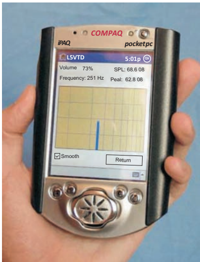
Fig. (10a). LSVTC with simple bar to indicate SPL and pitch from Matos et al. [33].
