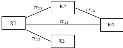
Fig. 2. A sample of a RIG in an AUTOSAR system.
