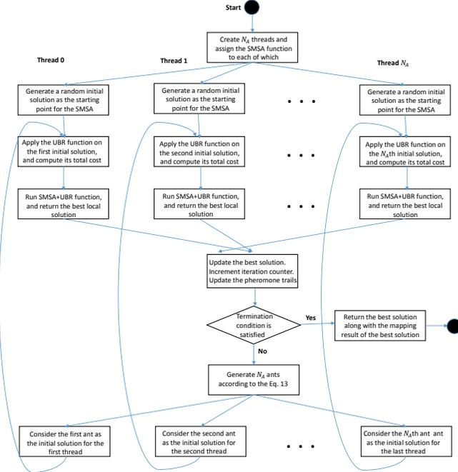
Fig. 4. Flowchart representation for the proposed solution framework.
