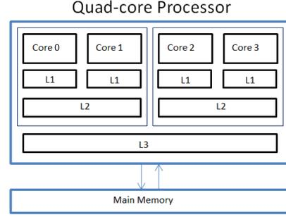
Fig. 3. A three-level shared-cache quad core architecture.
