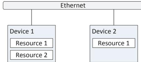
Figure 2.4: Example model of the platform in IEC 61499.
