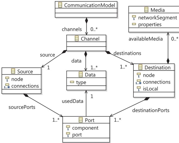
Figure 4.2: Ecore metamodel that defines the communication model.
