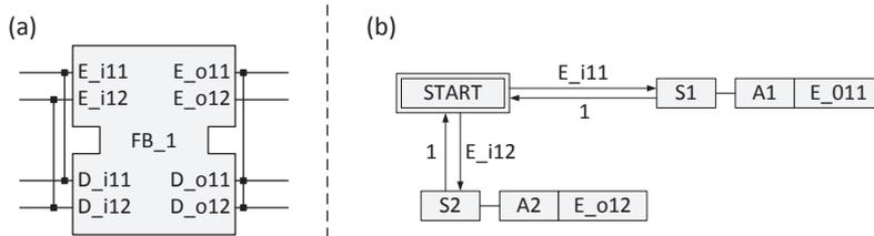
Figure 2.2: (a) An IEC 61499 function block interface. (b) A basic function block ECC.
