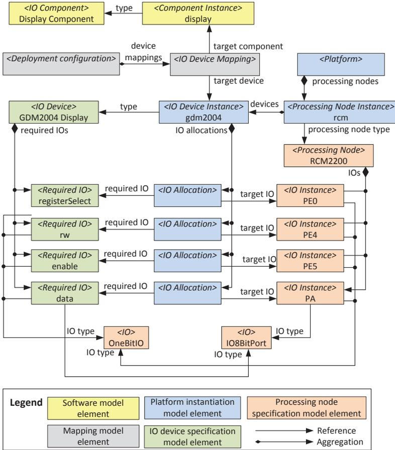
Figure 3.3: Example system, consisting of an IO component for display output, a GDM2004 display, and an RCM2200 microcontroller.
