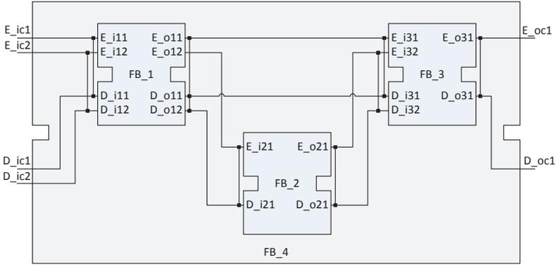
Figure 2.3: A composite function block with an internal function block network.
