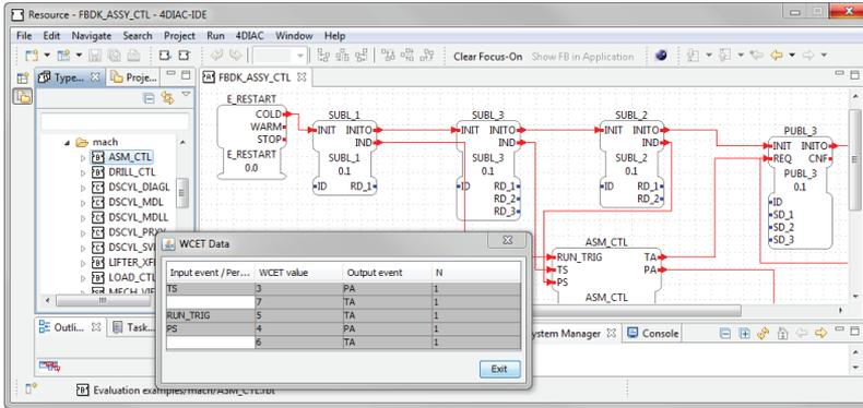
Figure 5.10: A screenshot of the 4DIAC tool showing results from the analysis plug-in.
