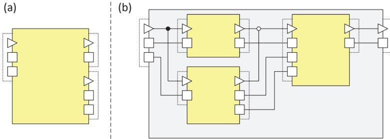
Figure 2.1: (a) ProSave component interface. The triangles and squares represent trigger and data ports, respectively. While the input ports are located on the left border of the components, the output ports are located on the right side. Port groups are denoted by dashed lines encompassing the ports. (b) An example of a composite ProSave component.
