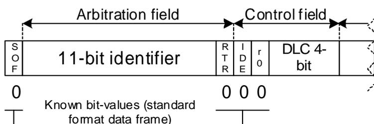
Figure 7.3: CAN frame header, the first 6 fields of the CAN frame (standard format).
