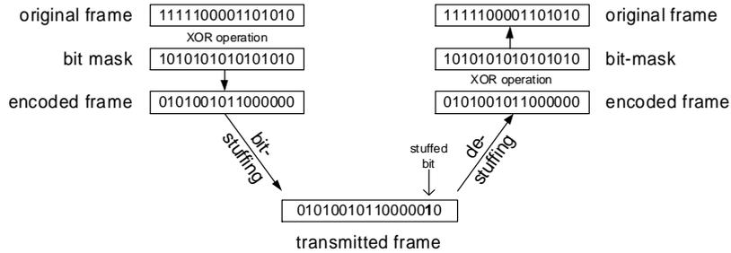
Figure 7.4: Encoding/decoding process for the proposed method.
