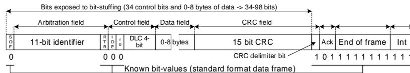
Figure 3.1: CAN frame layout (standard format data frame).
