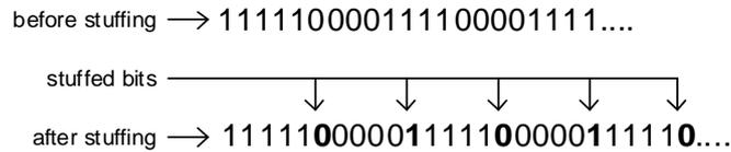
Figure 6.1: The worst-case scenario when stuffing bits.
