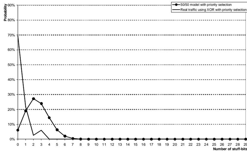
Figure 7.7: Probability density functions, PDF:s, showing the number of stuff-bits in a CAN frame (extended format). We show here real traffic manipulated with XOR and careful priority selecting. Our independent model is also shown with respect to the careful priority select.
