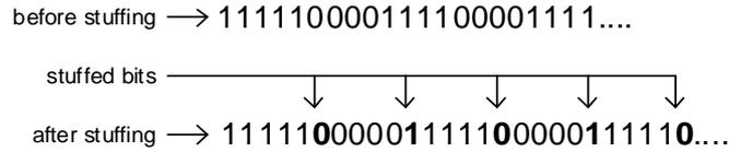
Figure 3.2: The worst-case scenario when stuffing bits.
