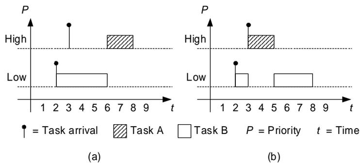
Figure 2.2: Task execution in a non pre-emptive (a) and a pre-emptive (b) system.
