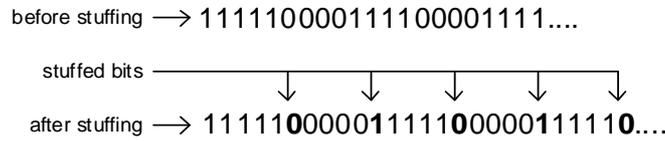
Figure 7.2: The worst-case scenario when stuffing bits.
