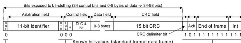
Figure 8.2: CAN frame layout (standard format data frame).
