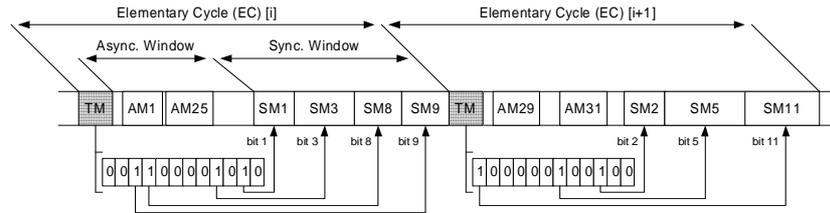
Figure 9.1: EC layout and TM data contents (FTT-CAN approach).
