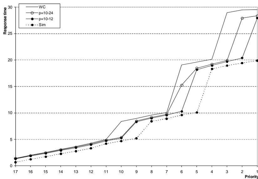
Figure 8.5: Message response-times (priority is the message ID as in Table 8.1).
