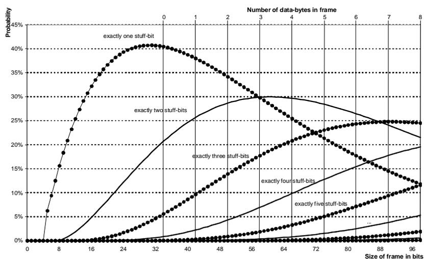
Figure 6.2: Probability of a specific number of stuff-bits in a frame, assuming our probabilistic frame model. The 9 frame lengths are marked as vertical lines.
