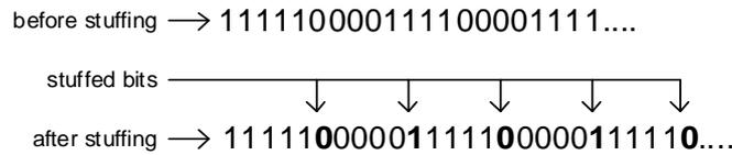
Figure 8.3: The worst-case scenario when stuffing bits.
