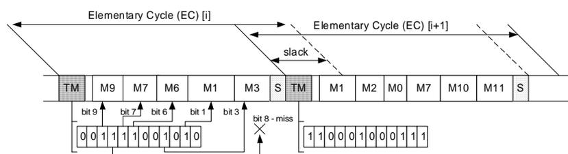
Figure 9.2: EC layout and TM data contents (server approach).
