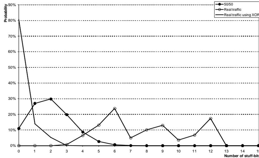
Figure 7.5: Probability density functions, PDF:s, showing the number of stuff-bits in a 64 bit frame. We show here our independent 50/50 model, the real CAN traffic and the manipulated real CAN traffic.
