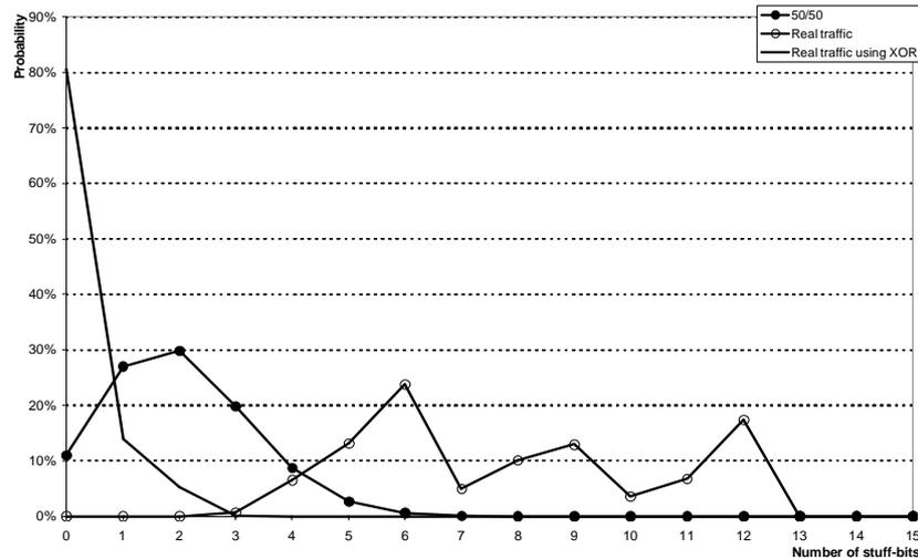
Figure 6.3: Probability density functions, PDF:s, showing the number of stuff-bits in a 64 bit frame. We show here our independent 50/50 model, the real CAN traffic and the manipulated real CAN traffic.
