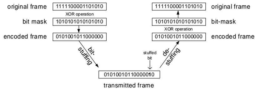
Figure 6.4: Encoding/decoding process for the proposed method.
