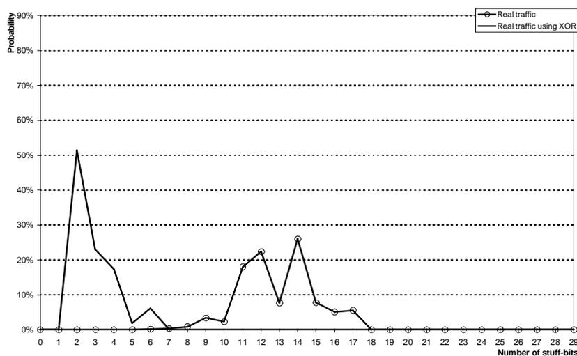
Figure 7.6: Probability density functions, PDF:s, showing the number of stuff-bits in a CAN frame (extended format). We show here real traffic along with the same traffic but manipulated with XOR.
