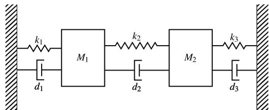
**Fig. 8** Separability parametric analysis of the double-mass, triple spring-damper system
