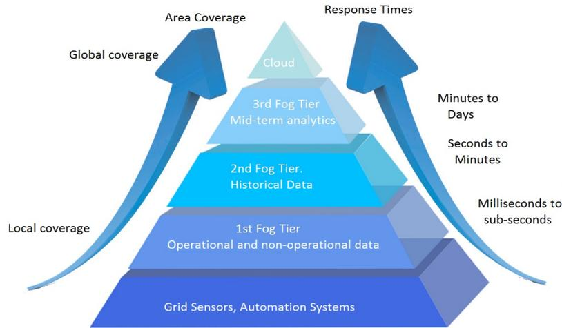
Fig. 1: A representation of the three-tier fog architecture by Cisco.
