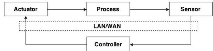
Fig. 3: Closed loop with networked controller.
