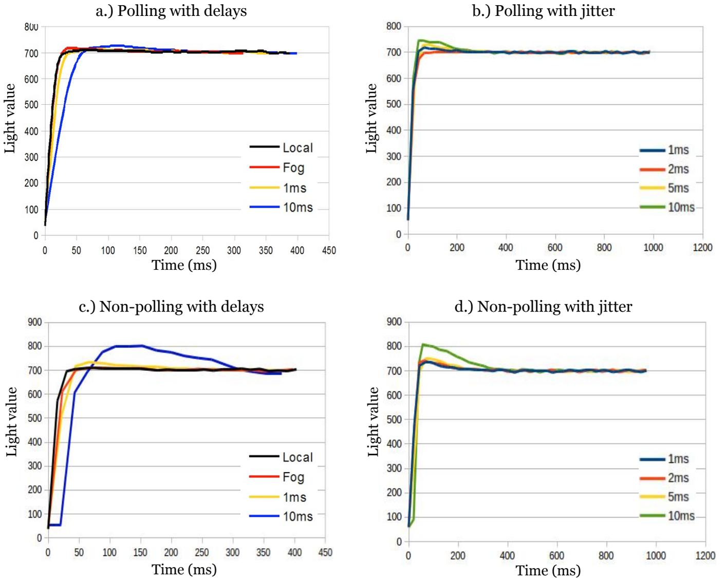
Fig. 5: System response under delay and jitter smaller than or equal to sampling period, both polling (a and b) and non-polling (c and d) approaches.
