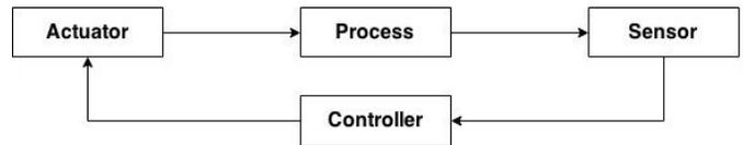
Fig. 2: Closed control loop.
