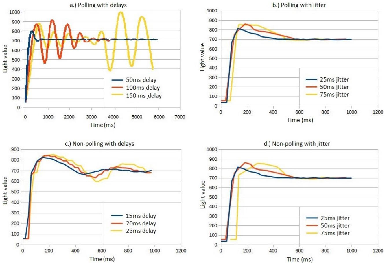
Fig. 6: System response under delay and jitter greater than sampling period, both polling (a and b) and non-polling (c and d) approaches.
