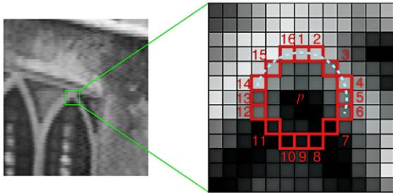
Fig. 1. FAST algorithm corner example where  $p$  is the currently selected pixel for analysis
