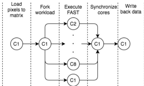
Fig. 3. FAST 8 core execution model
