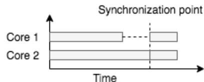
Fig. 4. Core idle issue due to synchronization
