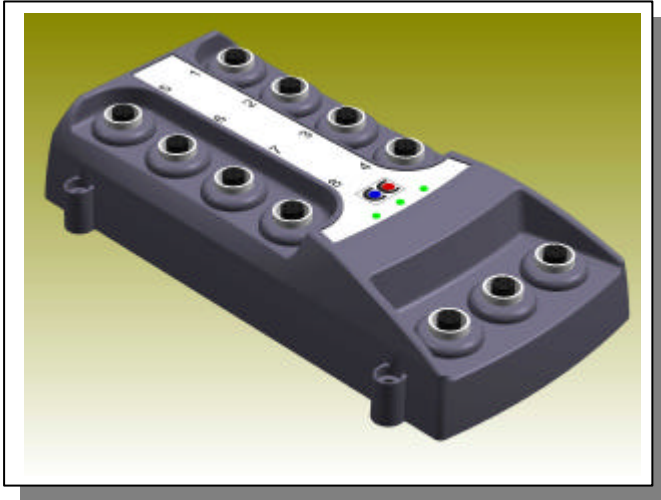
Figure 15: CC Systems IO distribution node, Cross Fire, used to test the CCOS API.
