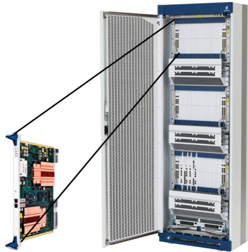
Figure 2.4: Many circuit boards (to the left) are interconnected to form a cabinet (to the right). Courtesy of Ericsson 2016.
