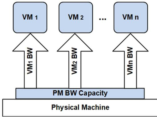
Fig. 2. The shared bandwidth for  $n$  VMs in one PM.
