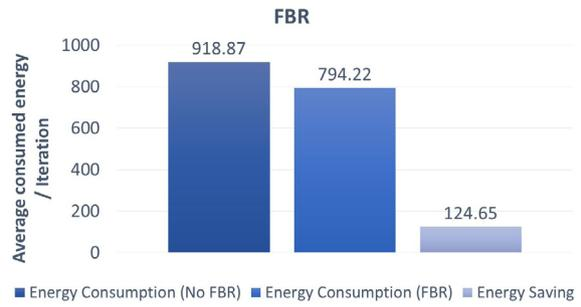
(b) Average energy consumption per emulation iteration by applying the FBR algorithm and the energy savings achieved.
