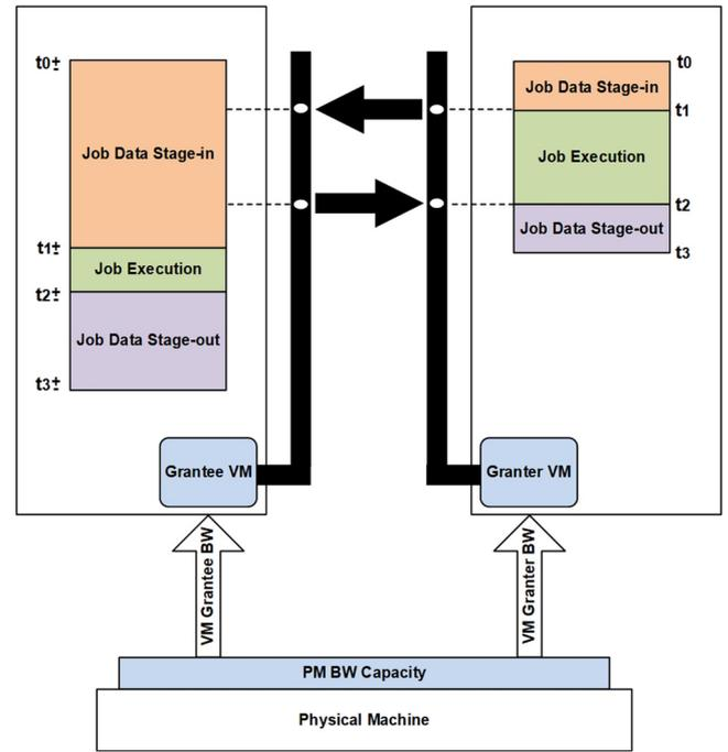
Fig. 4. The process of BW granting in the FBR Algorithm.
