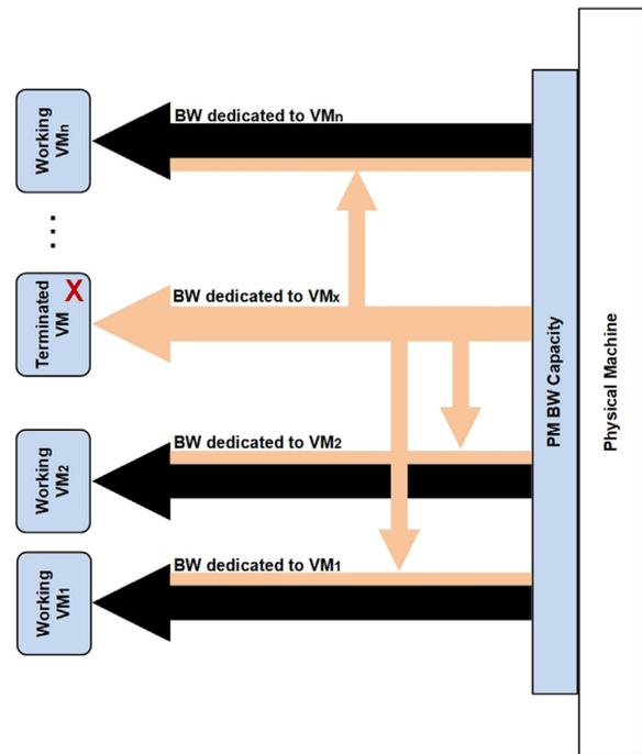
Fig. 6. The operations of the DBR algorithm.
