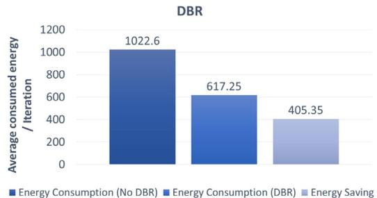
(b) Average energy consumption per emulation iteration by applying the DBR algorithm and the energy savings achieved.
