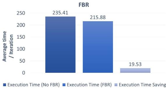
(a) Average execution time per emulation iteration by applying the FBR algorithm and the execution time savings achieved.
