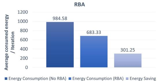
(b) Average energy consumption per emulation iteration by applying the RBA algorithm and the energy savings achieved.
