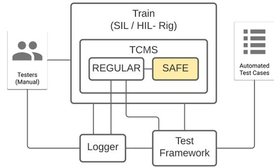
Fig. 1: Conceptual Overview, TCMS Testing Environment
