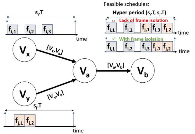
Figure 5: Frame isolation constraint.
