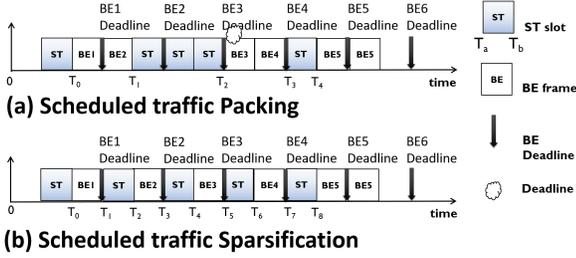
**Figure 6: Example of schedule bin-packing and the effect on schedulability of BE traffic.**
