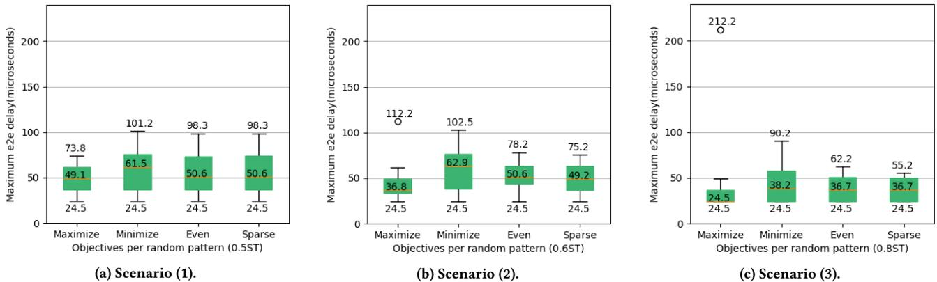
**Figure 10: Maximum end-to-end delays of the BE streams under various objective functions per traffic distribution case.**
