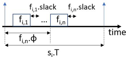
**Figure 7: Illustration of the proposed slack property of a frame per link.**
