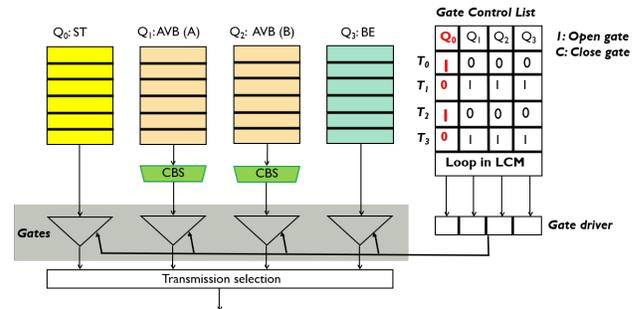
Figure 1: Gate mechanism block diagram.
