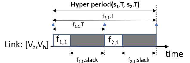
**Figure 8: The allowed range for slacks on a link.**
