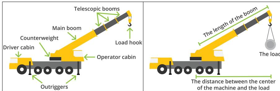
**Fig. 1.** The left image shows some parts of mobile cranes that are relevant to know in this paper. The right image shows the concepts of boom length and load radius in mobile crane operations.
