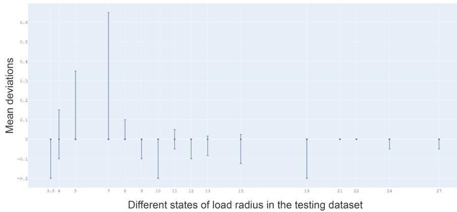
**Fig. 4.** The mean deviations of the predicted lifting capacity based on various states of load radius in the testing dataset. The x-axis shows whether the deviations were higher or lower than the values from the load charts. The y-axis shows the mean deviations of the predicted lifting capacity for each state of load radius.
