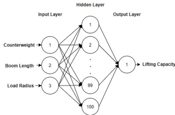
**Fig. 3.** The structure of the ANN that we used to predict the real-time lifting capacity. The prediction was made based on which counterweight configuration being used and the current states of boom length and load radius.
