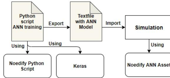
**Fig. 2.** The process of exporting and importing the trained ANN model from Keras to the simulation.
