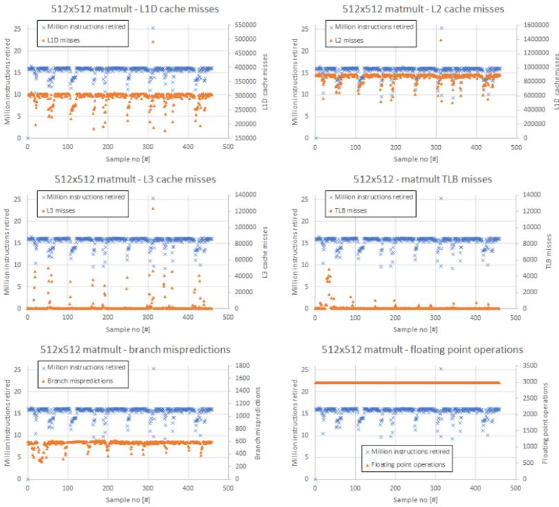
**Figure 8.3:** Execution characteristics of a 512x512 matrix multiplication
