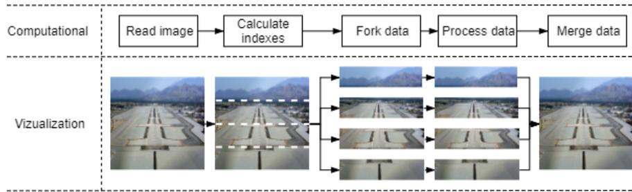
**Figure 7.3:** The image data is partitioned to support the fork-join model.
