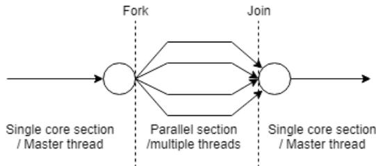
**Figure 7.2:** The fork-join model for parallelization of algorithms.
