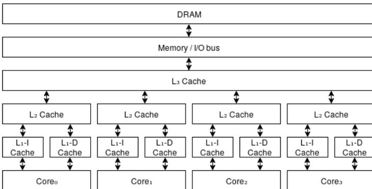
Figure 1.1: Example of a typical common 4-core system
