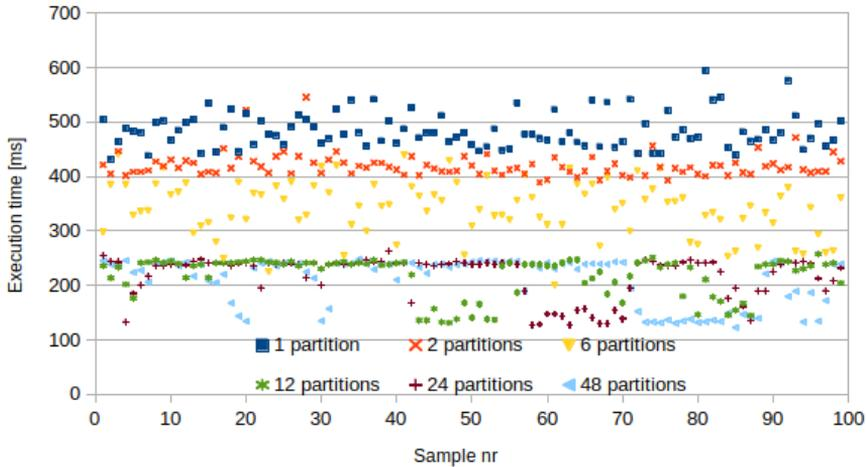
**Figure 12.3:** Matrix multiplication using different cache partition sizes
