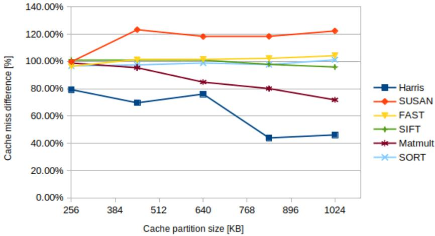
**Figure 9.9:** Difference in instructions retired misses using different  $L_2$ -cache partition sizes.
