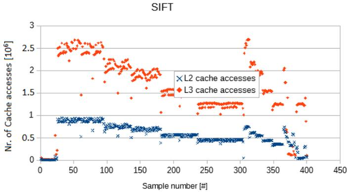
**Figure 13.5:** Memory usage illustration of SIFT using an 8MB image.
