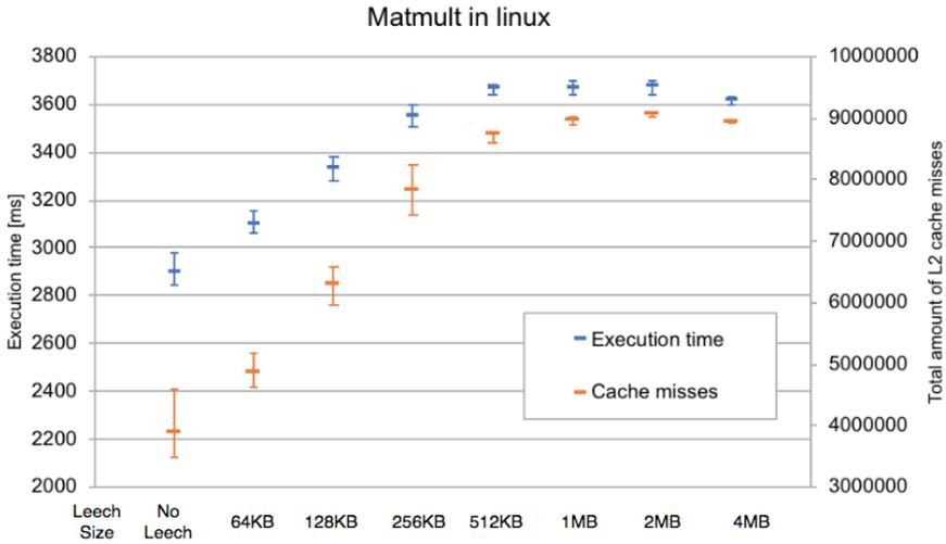
**Figure 10.3:** Linux L<sub>2</sub>-cache isolation test
