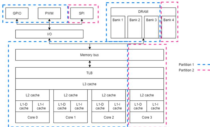
**Figure 2.11:** Example of a completely partitioned system
