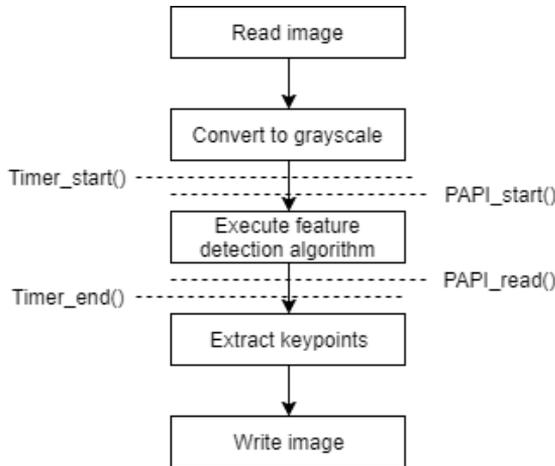
**Figure 7.4:** The algorithm performance measurement sequence.
