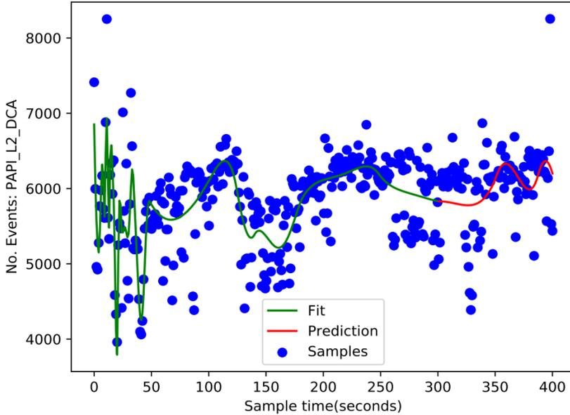
**Figure 13.4:** Example of an L<sub>2</sub> cache usage function estimated using a MARS model [19].
