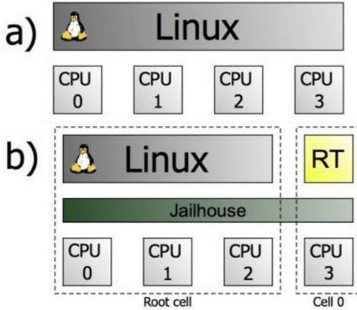
**Figure 10.1:** a) Usual Linux deployment. b) Linux with Jailhouse configuration [15].
