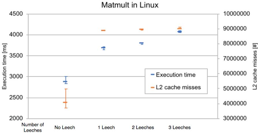
**Figure 10.5:** Linux memory bus isolation test
