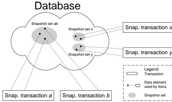
Figure 5. Snapshot sets in 2V-DBP-SNAP
