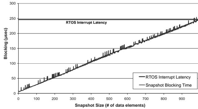
**Figure 8. Blocking introduced by soft transactions caching a snapshot set**
