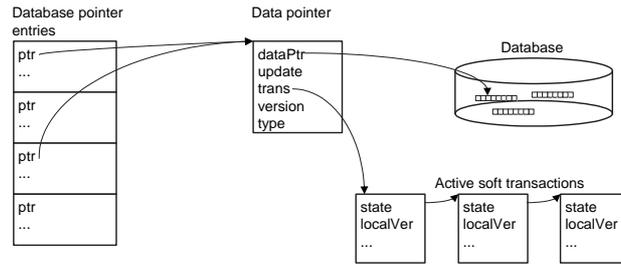
**Figure 2. The data structures used by database pointers under 2V-DBP.**
