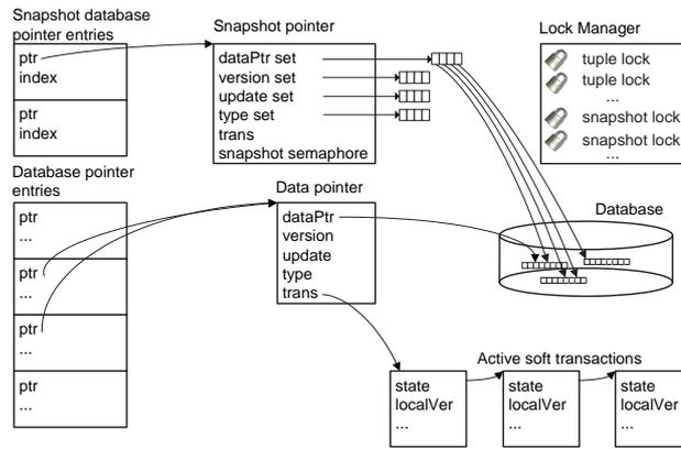
Figure 6. The extended data structures used by 2V-DBP-SNAP.
